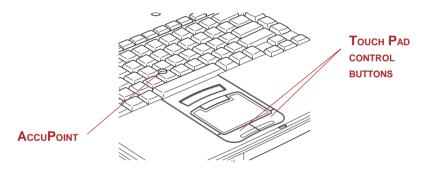
Figure 4-1 Touch Pad and Touch Pad control buttons
